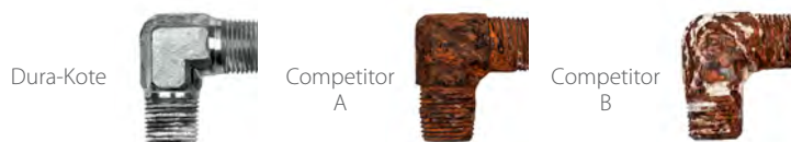
Corrosion comparison after 650 hours of exposure to salt spray testing.
